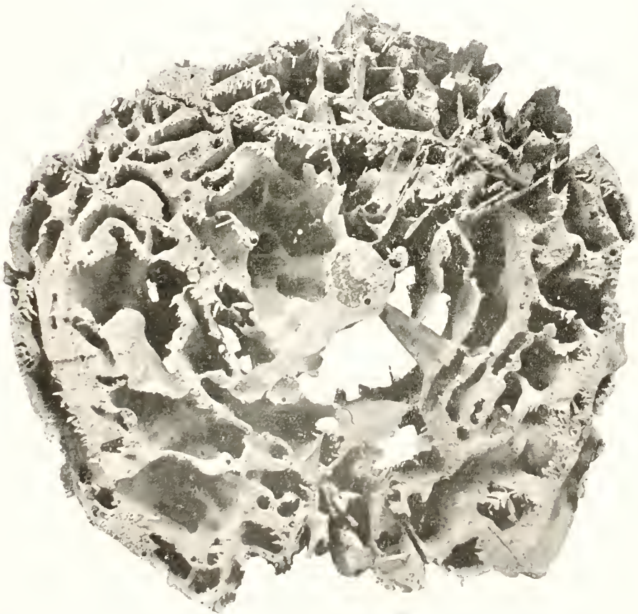
FIG. 37. Damage by Calotermes hubbardi to rafters in an "adobe" building in Arizona. (After Thos. E. Snyder.)
